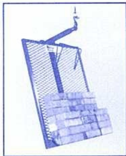
BRICK FORK 400 lb. capacity 29-1/4"L x 7-1/2"W x 37-1/2"H Max. brick size: 2-1/2" x 3" x 8"
